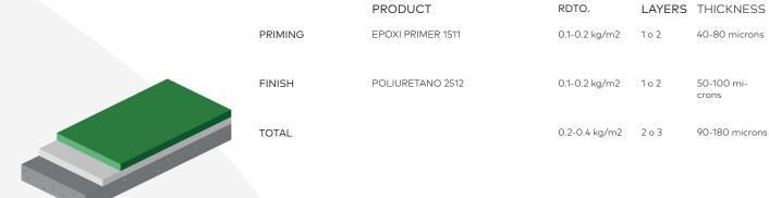
Note: These data are theoretical and do not take into account additional material costs due to porosity, roughness, losses, etc.
